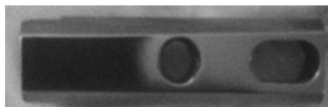
Figure 1. Component of the Ti6Al4V alloy hot forged
