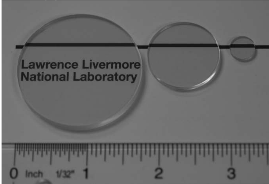
Figure 3. Photograph of \text{Lu}_2\text{O}_3 -based transparent ceramics. The fabrication method described herein allows increased part size while maintaining the high degree of transparency.
