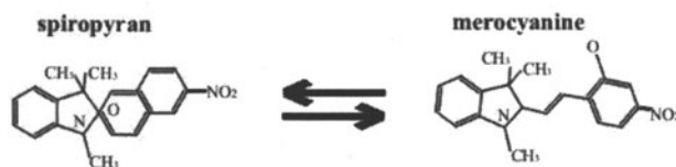
Figure 1. Schematic molecular structure of the sample before the UV illumination and after the isomerization. The process is reversible under visible illumination.
