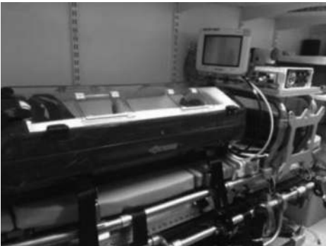
Figure 3.2 Baby pod secured to air stretcher. (A black and white version of this figure will appear in some formats. For the colour version, please refer to the plate section.)
