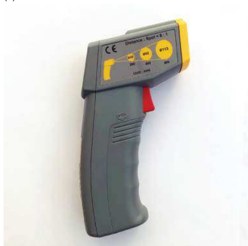
Figure 1.3. Different types of thermometers. (a) In a thermograph, a bimetallic strip bends and moves a pen up and down while a roll of paper turns underneath. (b) In a digital thermometer, the electrical resistance of a thermistor changes with temperature. (c) In an infrared thermometer, the radiation emitted by bodies is used to infer their temperature.
