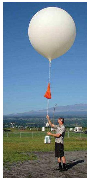
Figure 1.5. Radiosonde being launched in Hawaii.
