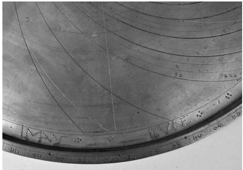
Figure 1.3 Detail from the womb of Wh.1264, showing the equator, almucantars, and unequal hours, and a finer Great House line (with corrected '6'). Note also the hammered-in month names and diamonds. Image © Whipple Museum.
