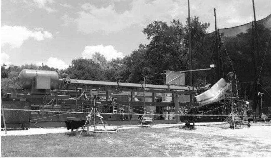
FIGURE 1.2. The large gas gun at SwRI. A cylindrical pressure vessel is to the left, followed by a fast-acting valve, followed by a long barrel. This photograph was taken before an impact test against the space shuttle leading edge test article, July 2003. High-speed cameras and lights surround the target.
