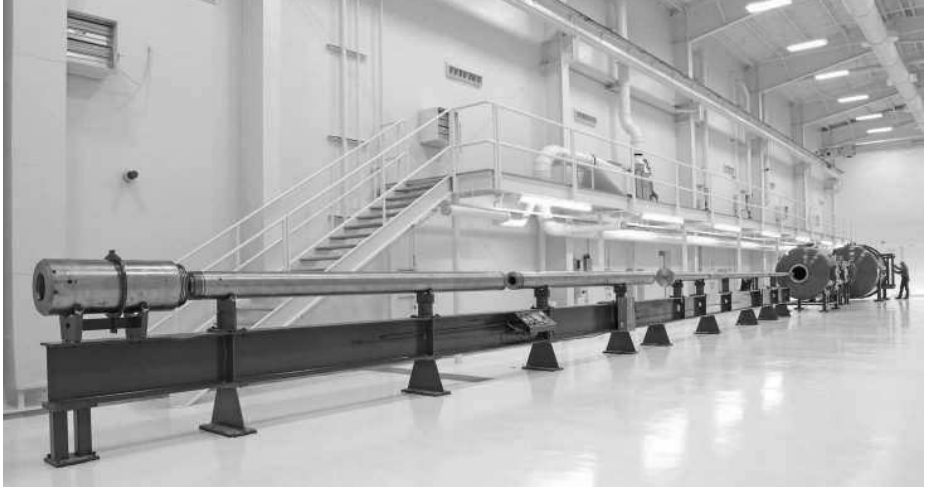
FIGURE 1.4. Large two-stage light gas gun at SwRI during assembly. The high pressure powder breech is to the left; the pump tube is in two parts; the high-pressure section connector is missing. Then come the launch tube and finally the evacuated target chambers. The gun can launch 60 grams to 7 km/s.
