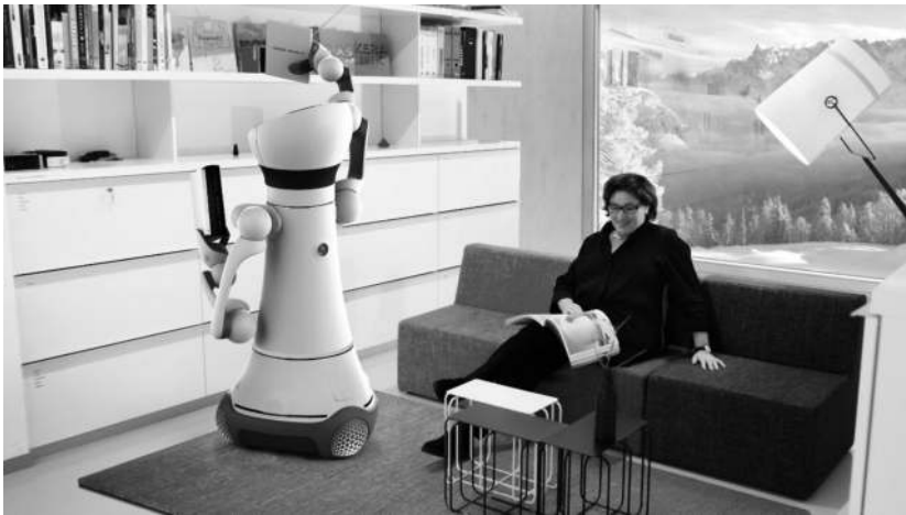
Figure 1.3 Care-o-Bot 4 robotic home assistant Source: Fraunhofer IPA: www.care-o-bot.de/en/ . Used with permission
