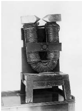
The large horseshoe electromagnet used by English physicist and chemist Michael Faraday, around 1830.
