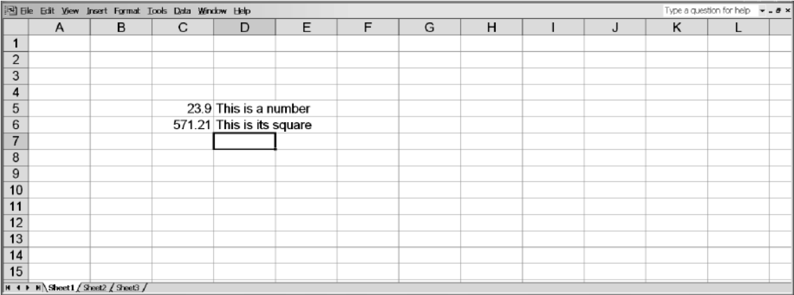
Figure III. Cell C6 carries the formula =C5*C5 and hence displays the square of 23.9.
