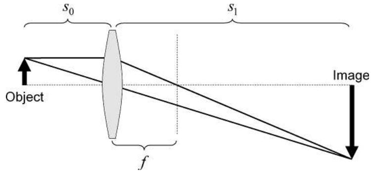
Figure 1.4. Imaging with a lens of focal length  $f$ .
