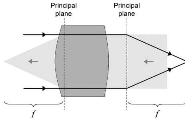
**Figure 1.5.** Principal planes of a thick lens of focal length  $f$ .
