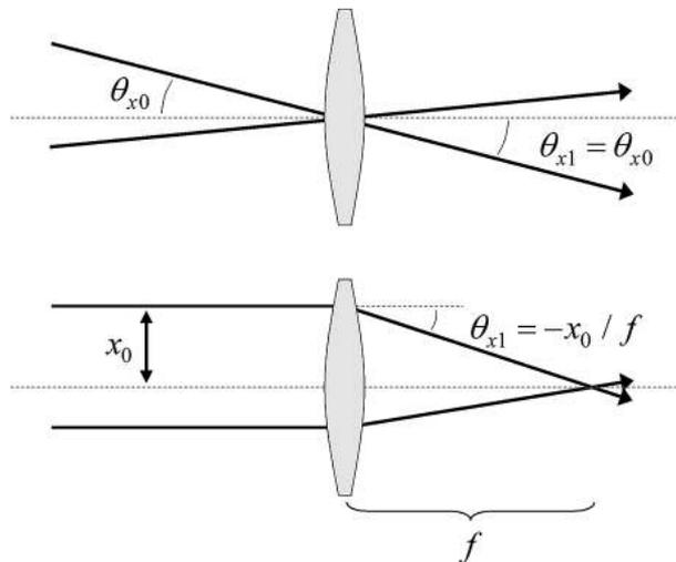
**Figure 1.3.** Propagation of rays through a lens of focal length  $f$ .
