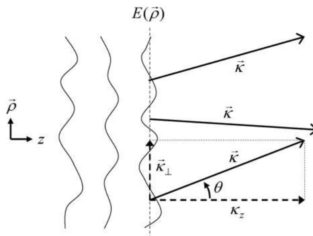
**Figure 1.1.** Connection between wave optics and ray optics.
