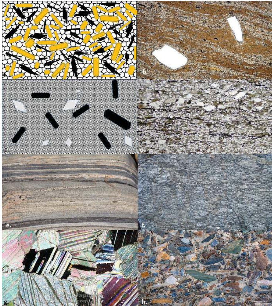
Figure 1.5 (a) Fabric or texture of granite rocks as an example of plutonic rocks. Even-grained crystals without preferred orientation: feldspars are uniform yellow; mica shows close parallel black plates; white in the remaining space is quartz. Especially, feldspars form idiomorphic crystals, while quartz is xenomorphic. (b) Fluidal texture in volcanic rocks. Crystals follow in their arrangement the flow pattern of melt. (c) Porphyritic structure of igneous rocks. Crystals float in a fine-grained crystalline matrix. Large crystals had already been formed within the magma chamber. After a rapid deflation of the chamber, they were transported upwards together with melt during a volcanic eruption; this itself causes fast cooling and, therefore, results in a finely crystalline or even glass-like solidified host matrix. (d) Structure of clastic sediments. Quartz is rounded and white, mica is of an almost parallel orientation and dark, while feldspar is grey. (e) Parallel texture of gneiss as an example of metamorphic rocks. (f) Texture in eye gneiss. (g) Puzzle-like arrangement of calcite crystals in metamorphic marble rock showing twinning planes. (h) Breccia texture consisting of different rock fragments randomly cemented or compressed together inside finer-grained host material.
