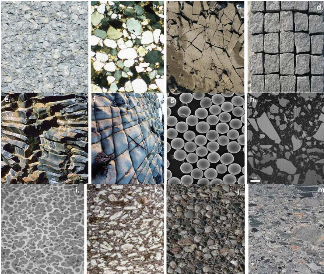
Figure 1.3 Classification of main rock textures: a – crystalline; b – clastic-round grain, c – clastic-angular; d – cubic; e – columnar; f – parallelepiped; g – uniform; h – continuous nonuniform; i – discontinuous nonuniform; k – porphyritic; l – conglomerate; m – breccia.
