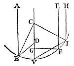
all cases, therefore if the radii C B, C F be drawn to the points of incidence, and thence BD making the angle CBD equal to the angle CBA, and FG making the angle CFG equal to the angle CFE; then BD, FG will be the reflected rays, and D, G, the points where
