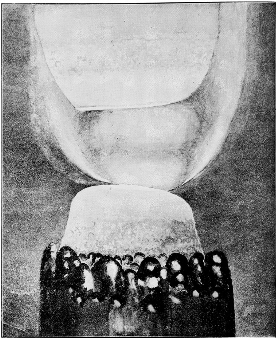
FIG. 5. —Carbons: Positive, 18mm. cored; Negative, 15mm. solid. Current, 20 amperes. P.D. between Carbons, 51 volts. Length of Arc, 7mm.
