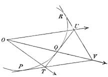
force into two components which act along TP and TQ. It follows that the resultant force on any arc PQ may be balanced by two forces or tensions acting along the tangents at P and Q.
