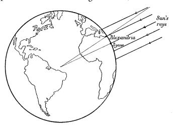
Fig. 1. Eratosthenes found that when the sun's rays fell vertically at Syene, they were a fiftieth of a whole circle away from the vertical at Alexandria. He concluded that the circumference of the earth was fifty times the distance from Alexandria to Syene.
