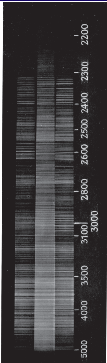
Fig. 2. Spectrogram of iron arc.
