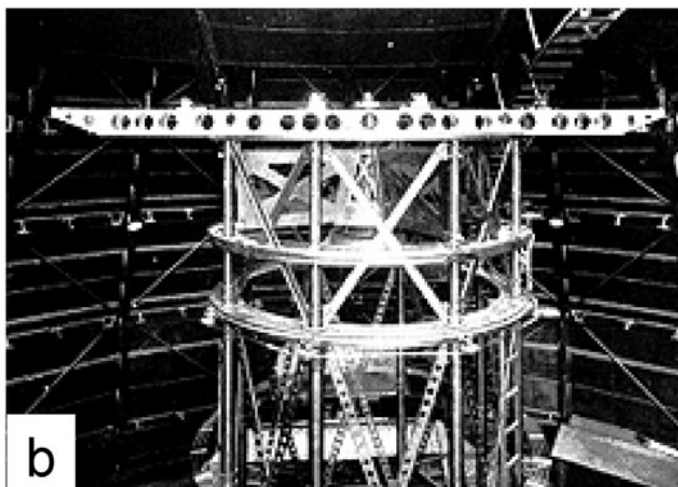
Fig. 1.2. Michelson's 20-foot beam stellar interferometer. (a) Optical diagram; (b) a photograph of the instrument, as it is today in the Mount Wilson Museum (reproduced by permission of the Huntington Library).
