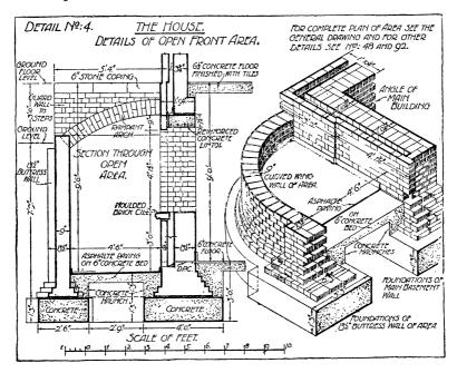
being a rectangle with two quadrant ends, the rectangle lying beneath the main entrance steps with the quadrants open to view and forming wing walls to the excavation.
