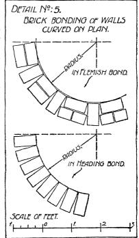
ible and the bricks must then be rough-axed to a wedge shape, or purpose made bricks obtained.
