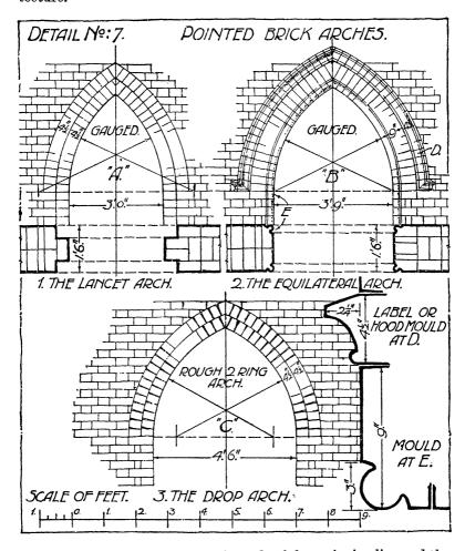
Forms of pointed arch. When the ends of the springing line and the crown of the arch lie upon the angles of an equilateral triangle, the arch is named "equilateral"; to describe the intrados curve the centres are at the ends of the springing line and the radius is equal to the span.
