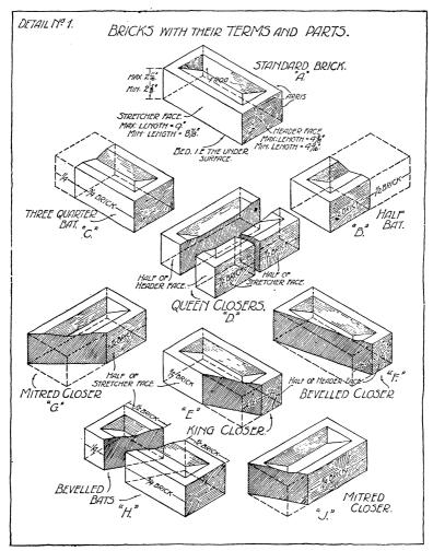
"King closer"—a brick reduced to a width of  $2\frac{1}{4}$ " at one end by cutting off the triangular piece between the centre of one end and the centre of one side.—Detail 1 E.
