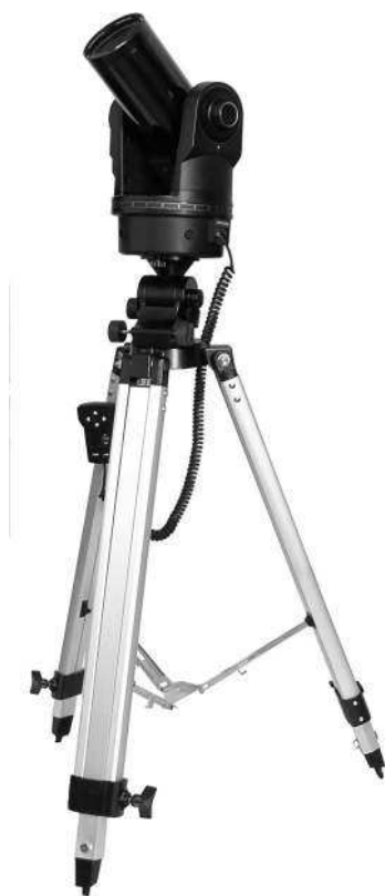
Figure 1.8 A widely used, intermediate-level telescope. With a compact design, a light weight, a motorized mount, and stable, good optics, it delivers very sharp images given the aperture.
