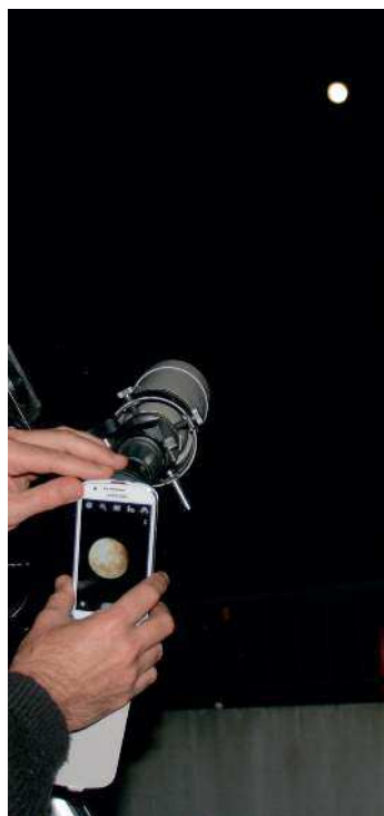
Figure 1.5 Shooting with a smartphone held by hand behind a small refractor equipped with an 8-mm eyepiece. The mount was undriven (like a simple, sturdy photo tripod). Image by Catherine Port.
