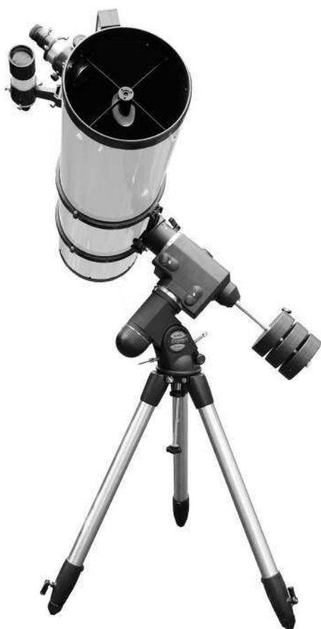
Figure 1.10 A 200–300-mm (8–12-in) Newtonian telescope or a 250–280-mm (10–11-in) Schmidt–Cassegrain telescope resolves 600-m details. This is a portable but cumbersome and heavy instrument, typically weighing about 30–50 kg (66–110 lb).
