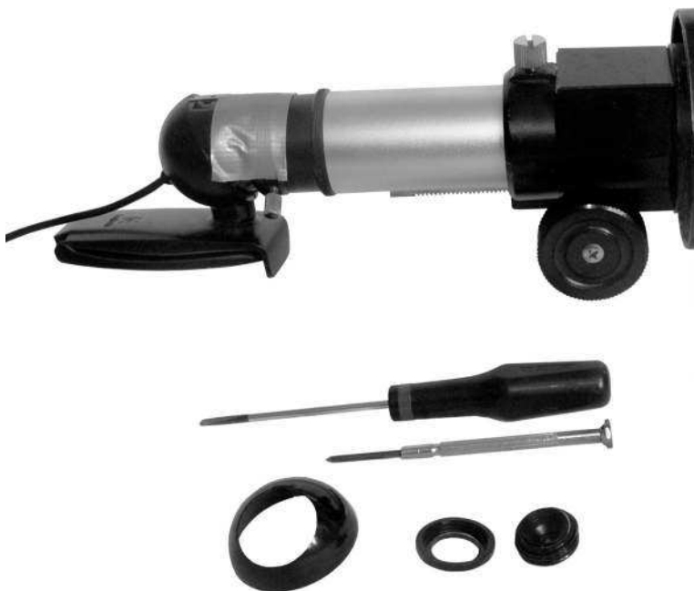
Figure 1.7 The housing of the webcam is partially removed to unscrew its lens (the plastic housing is fragile and opening it voids the guarantee). Then the webcam, with its bare sensor, is attached to a small refractor with no eyepiece with the help of heavy-duty, opaque adhesive tape. The refractor is placed on a stable video tripod, allowing you to acquire decent still images, although the tripod cannot compensate for the diurnal motion.
