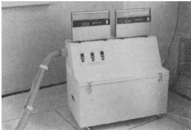
Fig. 1.8 The controller of the forced-air warmer used by Lewis. (Reproduced from: Lewis RB, Shaw A, Etchells AH. Contact mattress to prevent heat loss in neonatal and paediatric surgery. Br J Anaesth 1973; 45 : 919–922 [13] with kind permission of Oxford University Press.)
