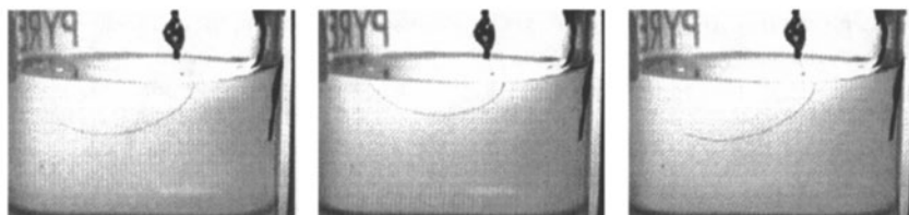
Figure 4. Electromechanical actuation of a SWNT fiber in an electrolyte solution (NaCl 1M) when an AC voltage of 1V is applied at a frequency of 1Hz. To make a simple bimorph device, the fiber is coated on one side with a polymer gel that doesn't respond to the applied voltage. In contrast, the nanotubes expand and contract upon charge injection as described in reference 7. As a result the bimorph exhibits a periodic motion as shown in the pictures.
