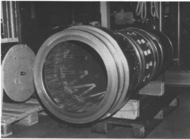
Fig. 3: Laser hardened diesel cylinders 750 mm id., MAN München photograph
