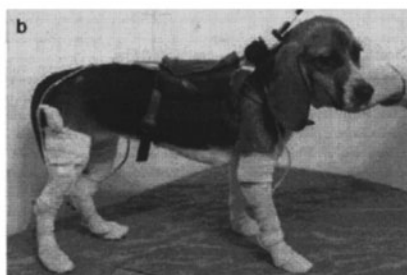
Figure 7. Cellular polypropylene sensor element for detecting forces acting upon dog limbs [20].
