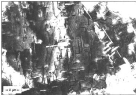
Figure 5. TEM plan view image of thinned 1 μm thick Cu-Co alloy film after annealing [25].
