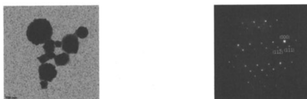
(a) TEM photographs of produced powder. (b) Selective diffraction pattern of single particle.
