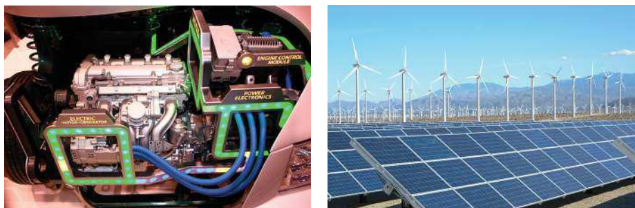
FIGURE 1.1 Examples of energy conversion systems: Hybrid engine converts energy stored in chemical bonds of fuel molecules or from batteries to shaft power (left) (GreenPimp / E+ / Getty images); photovoltaic solar panels and wind turbines convert solar radiation and wind energy to electricity, respectively (right) (GPhotoStock / Cultura / Getty Images).
