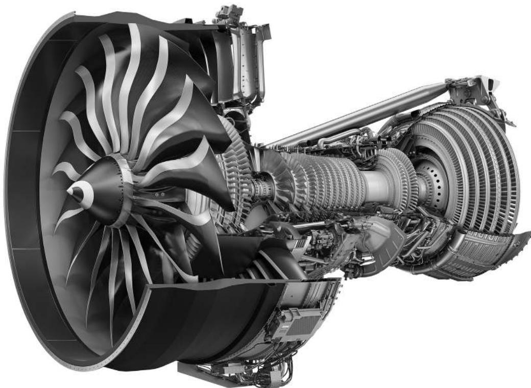
**Figure 1.1** Cutaway view of the GE9X engine (with permission from GE Aviation).
