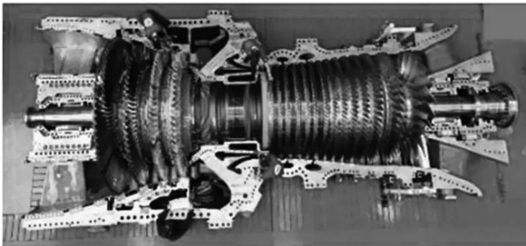
**Figure 1.2** Cutaway view of GE's 9HA gas turbine (with permission from GE).
