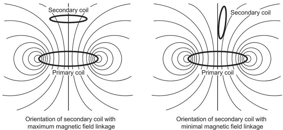
**Figure 1.5** Orientation of the secondary coil.
