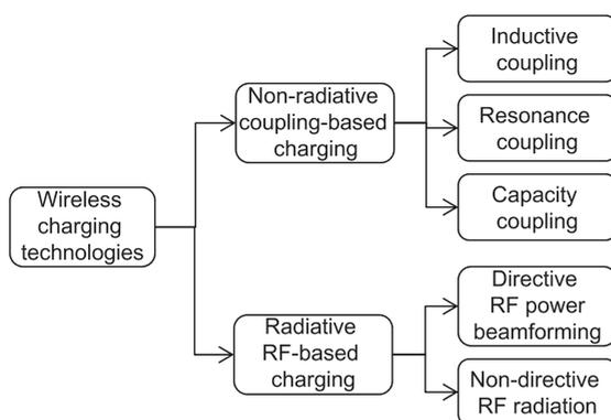
**Figure 1.2** Classification of wireless charging technologies.
