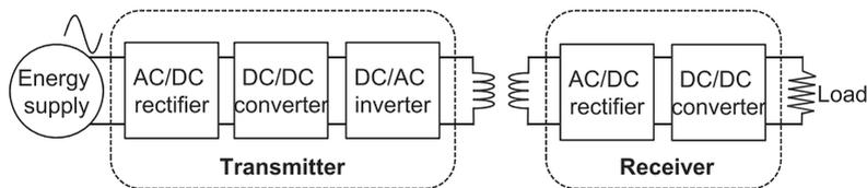
**Figure 1.3** Major components of a non-radiative wireless energy transfer system [8].
