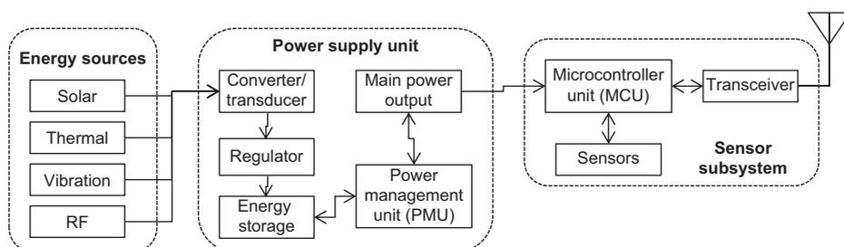
**Figure 1.1** A generic model of an energy harvesting sensor device [1].
