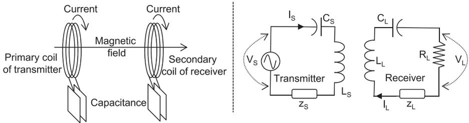
**Figure 1.6** Magnetic resonance coupling.
