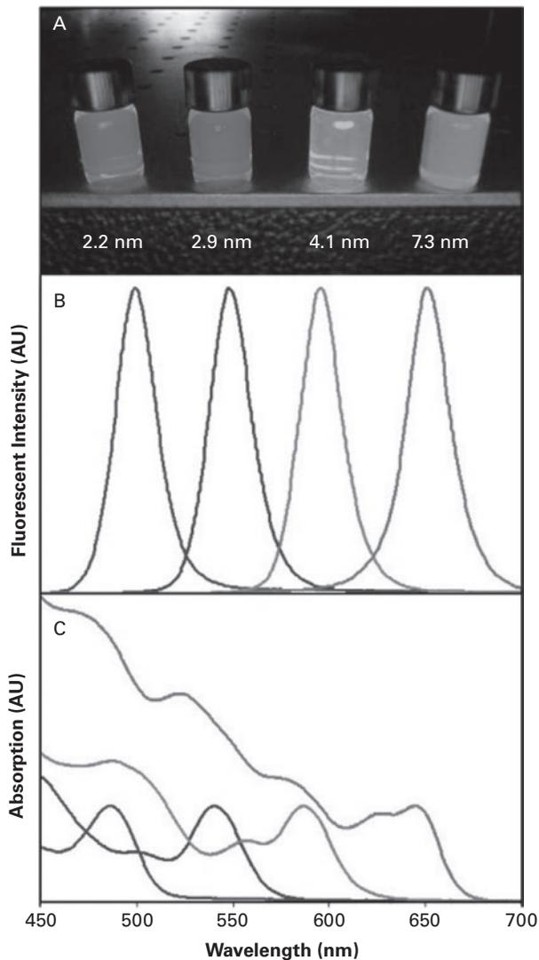
**Figure 1.4** Size-dependent optical properties of cadmium selenide QDs dispersed in chloroform, illustrating quantum confinement and size-tunable fluorescence emission.
