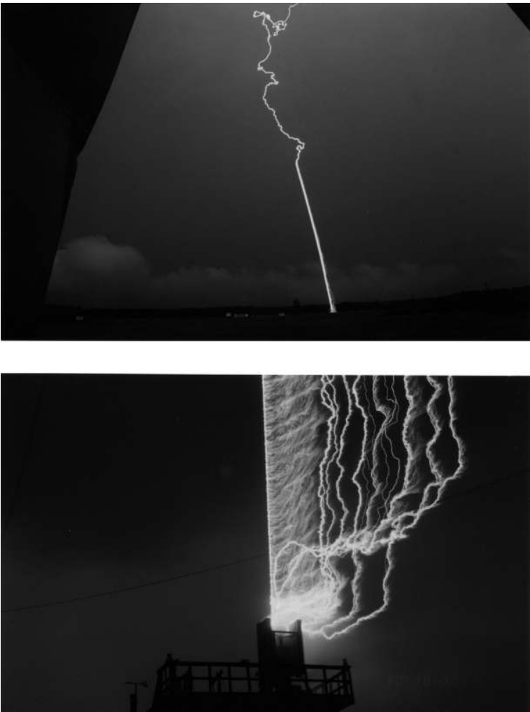
Fig. 1.7 Photographs of lightning flashes triggered using the rocket-and-wire technique at Camp Blanding, Florida. Top – a distant view of a strike to the test runway; bottom – a close-up view of a strike to the test power system. © Vladimir A. Rakov and Martin A. Uman 2003, published by Cambridge University Press, reprinted with permission.
