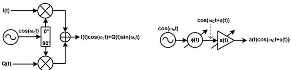
**Fig. 1.3** Direct generation of modulated waveforms using direct  $I/Q$  and polar transmitter architectures.
