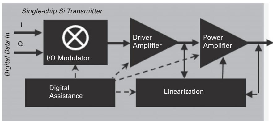
Fig. 1.4 Conceptual block diagram of an ELASTx silicon mm-wave transmitter SOC.
