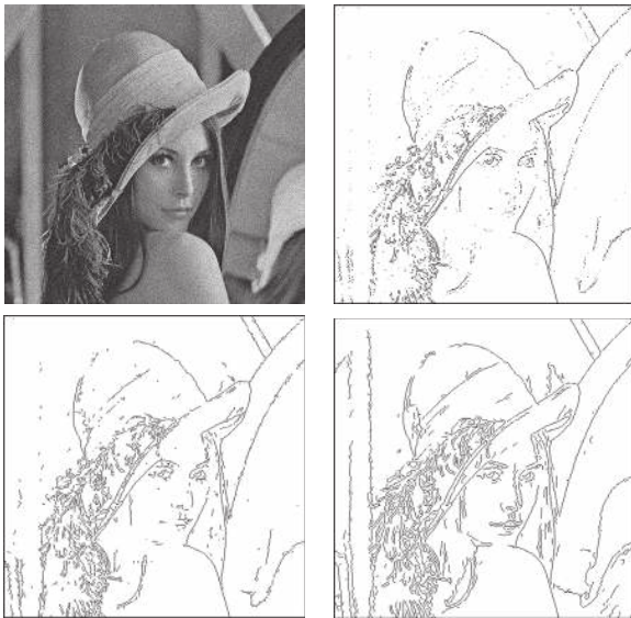
Figure 1.5 Edge detection results (clockwise from top to bottom): noisy Lena image; Sobel result; wavelet result; shearlet result.
