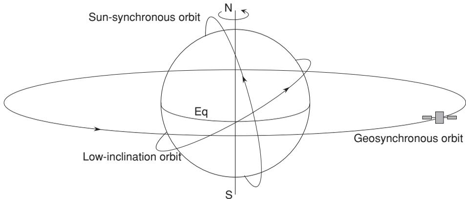
Fig. 1.3. Examples of the Sun-synchronous, geosynchronous and low-inclination orbits, where “Eq” is the equator. (Adapted from Asrar and Dozier (1994), Figure 3).
