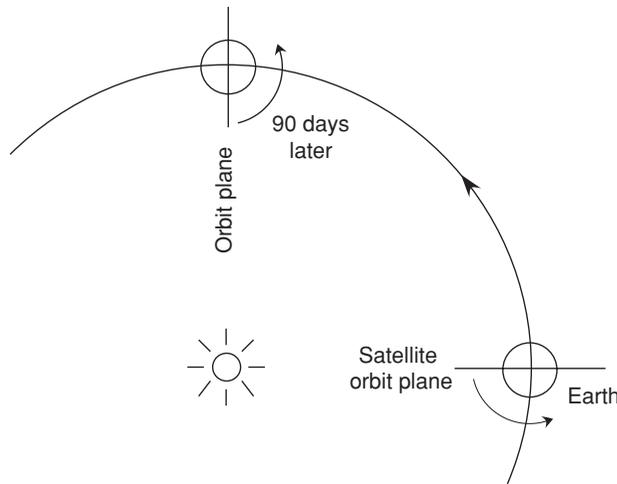
Fig. 1.4. Rotation of the plane of a Sun-synchronous orbit in the Earth–Sun orbit plane.
