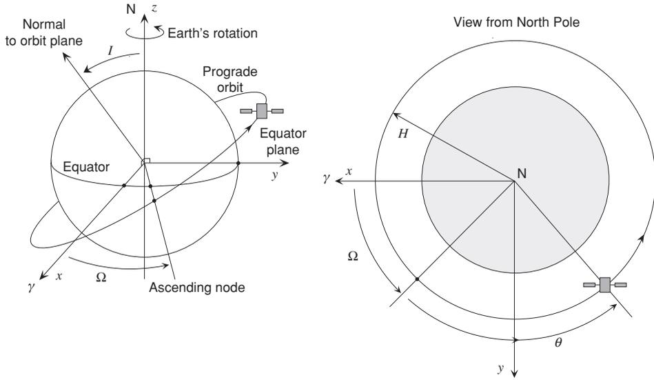
Fig. 1.1. For a circular orbit, the Keplerian parameters used to describe the orientation of the orbit plane and the satellite position along the orbit.
