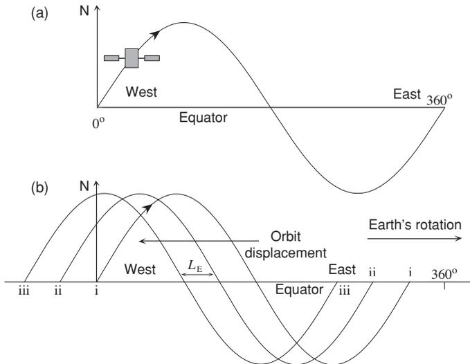
Fig. 1.2. Mercator map of the satellite ground track for the orbit shown in Figure 1.1 and for a (a) non-rotating Earth and (b) rotating Earth. See the text for further description. (Adapted from Elachi (1987, Figure B-6).
