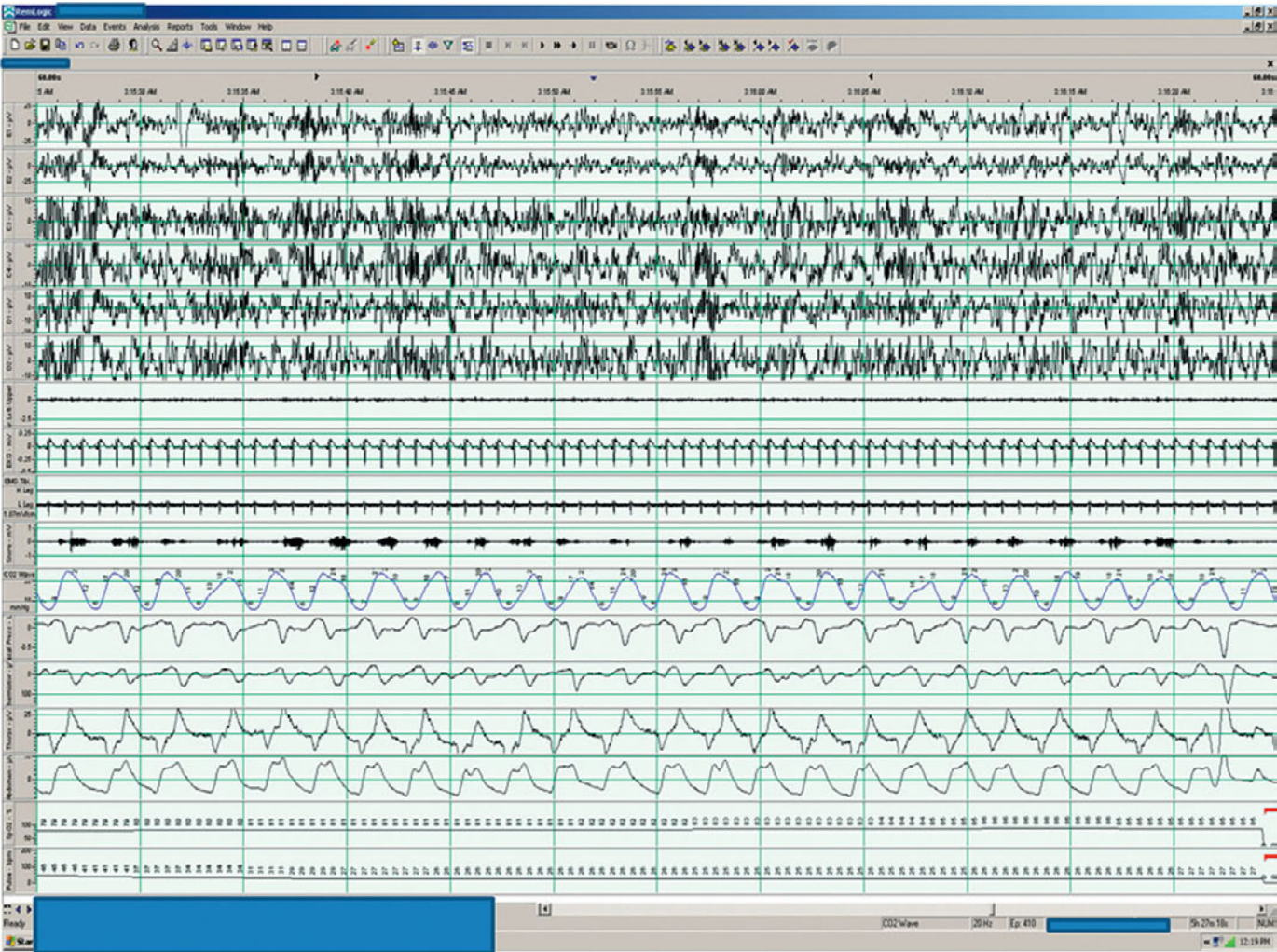
Abdomen, abdominal respiratory inductance plethysmography; CO2 wave, ETCO 2 ; Left-upper, submental EMG; Thorax, thoracic respiratory inductance plethysmography; SpO 2 by ear pulse oximetry. SpO 2 values are in the high 70 to mid 80% range (2nd channel from bottom). ETCO 2 (7th channel from bottom) is < 30mmHg throughout tracing. Pulse is displayed as the bottommost channel and shows values of ≤ 45bpm throughout the tracing.
