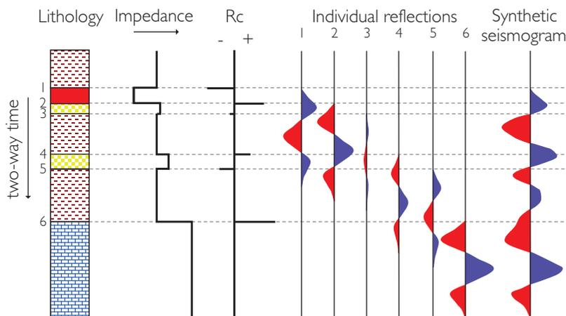
**Figure 2.7** Synthetic seismogram using a causal (i.e. recorded) wavelet with SEG standard polarity (re-drawn and modified after Anstey, 1982).
