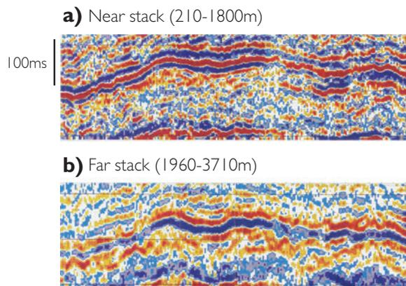
**Figure 2.4** Offset stacking example; (a) near stack, 210–1800 m offset, (b) far stack, 1960–3710 m offset. Note that the choice of offsets is dependent on the offset range available and the depth of the target. In this case the offsets have been selected to avoid stacking across a zone of phase reversal.
