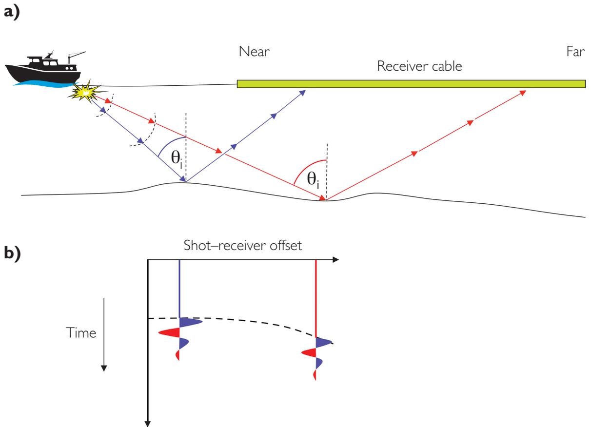
**Figure 2.1** Marine seismic geometry 1; (a) source and receiver configuration showing wavefronts, rays (perpendicular to wavefronts) and angle of incidence increasing with offset (b) a shot gather representation of the recorded energy. For a horizontal layered case the reflections form a hyperbola on the gather. Note that the amplitude of a reflection on the gather is related to the rock contrast across the boundary and the decrease in amplitude due to wavefront divergence.
