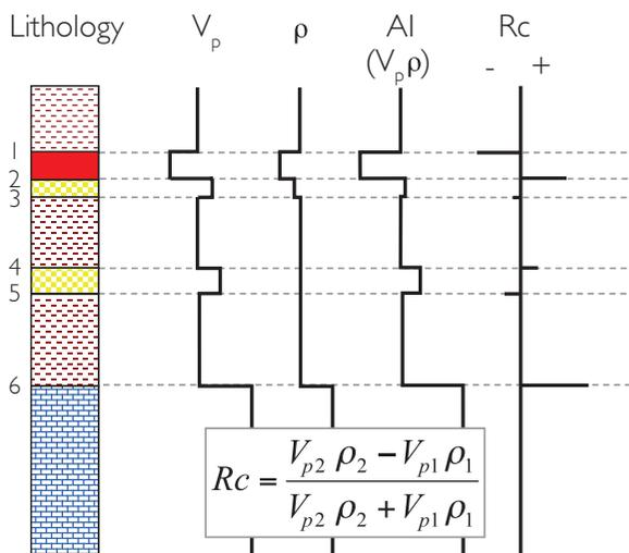
**Figure 2.6** The reflection coefficient as defined by the differentiation of the acoustic impedance log (re-drawn and modified after Anstey, 1982).
