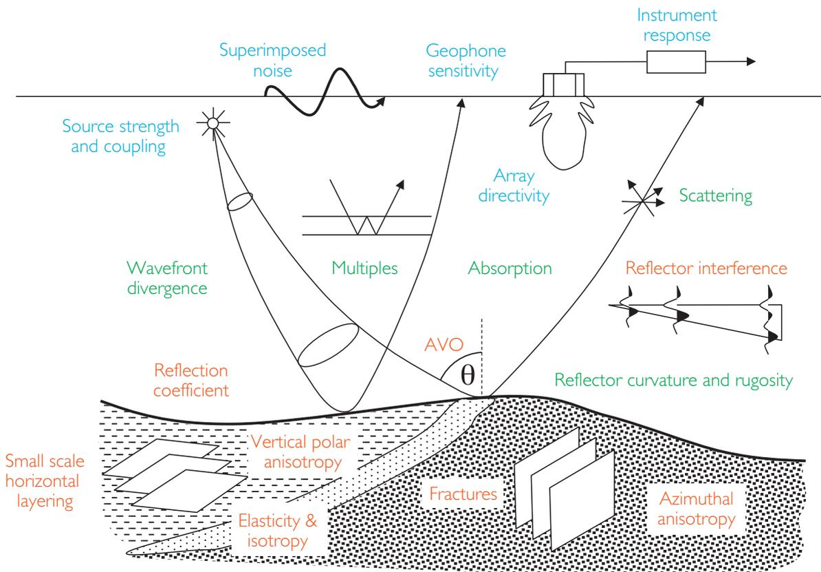
**Figure 2.5** Factors affecting seismic amplitude (modified after Sheriff, 1975).
