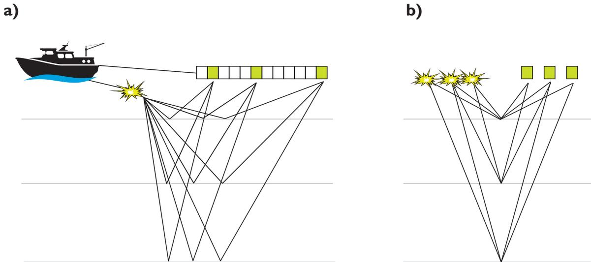
**Figure 2.2** Marine seismic geometry 2; (a) acquisition; each shot is recorded at a variety of receivers depending on the depth and the angle of reflection and (b) the common midpoint (CMP); if it is assumed that the Earth is flat the data can be arranged according to reflection location, i.e. different source–receiver pairs sampling the same position in the subsurface. For more complex velocity overburden sophisticated imaging solutions are required.
