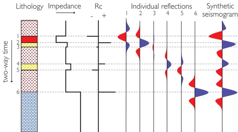
**Figure 2.9** Synthetic seismogram using a symmetrical wavelet with positive standard polarity (re-drawn and modified after Anstey, 1982). This illustrates the importance of zero phase to the interpreter; the main layer boundaries are more easily identified with the processed symmetrical wavelet compared to the recorded asymmetrical wavelet shown in Fig 2.7.
