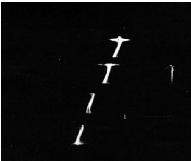
Figure 1.1 A cosmic ray detected in a four-gap spark chamber (Fukui and Miyamoto, 1959). By kind permission of Springer Science+Business Media.
