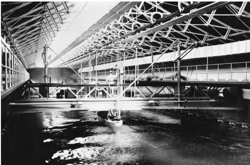
Figure 1b Model ship in towing tank
