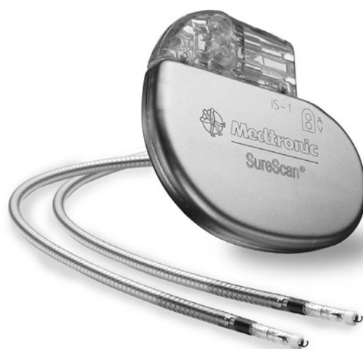
Figure 1.4 Cardiac pacemaker. Structure of an implantable cardiac pacemaker. The device has a chamber encased with titanium, two leads with electrode tips and a header through which the leads enter the chamber. This particular device has been designed to be MRI-compatible since many patients with pacemakers often require imaging and conventional pacemakers are not compatible with the magnetic fields used in MRI. Image courtesy of Medtronic Inc.
