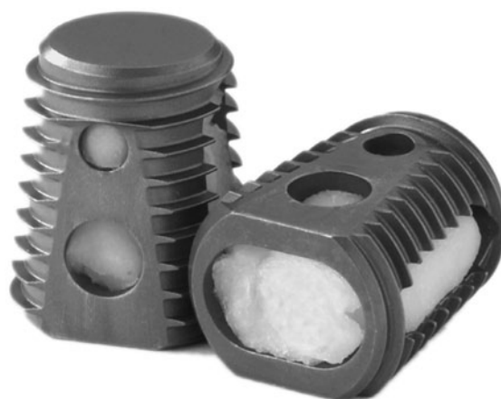
Figure 1.1 Device for spinal fusion surgery. The illustration shows an Infuse® Bone Graft with an LT-Cage® used in the lower part of the spine. This device consists of titanium cages that contain collagen sponge mixed with recombinant Bone Morphogenetic Protein-2 (BMP-2); this system incorporates technology developed by Gary K Michelson MD. Image provided by Medtronic, Inc.
