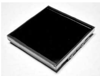
FIGURE 1.7. Fairchild CCD 4K × 4K, 15 μm pixels (left). The QE of modern CCDs can be made quite high, very nearly approaching 100% (right).
