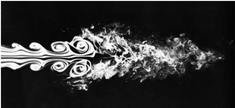
Figure 1.1 Instability of an axisymmetric jet. A laminar stream of air flows from a circular tube at the left at Reynolds number 10 000 and is made visible by a smoke wire. The edge of the jet develops axisymmetric oscillations, rolls up into vortex rings, and then abruptly becomes turbulent. Photograph courtesy Robert Drubka and Hassan Nagib. From Van Dyke (1982).
