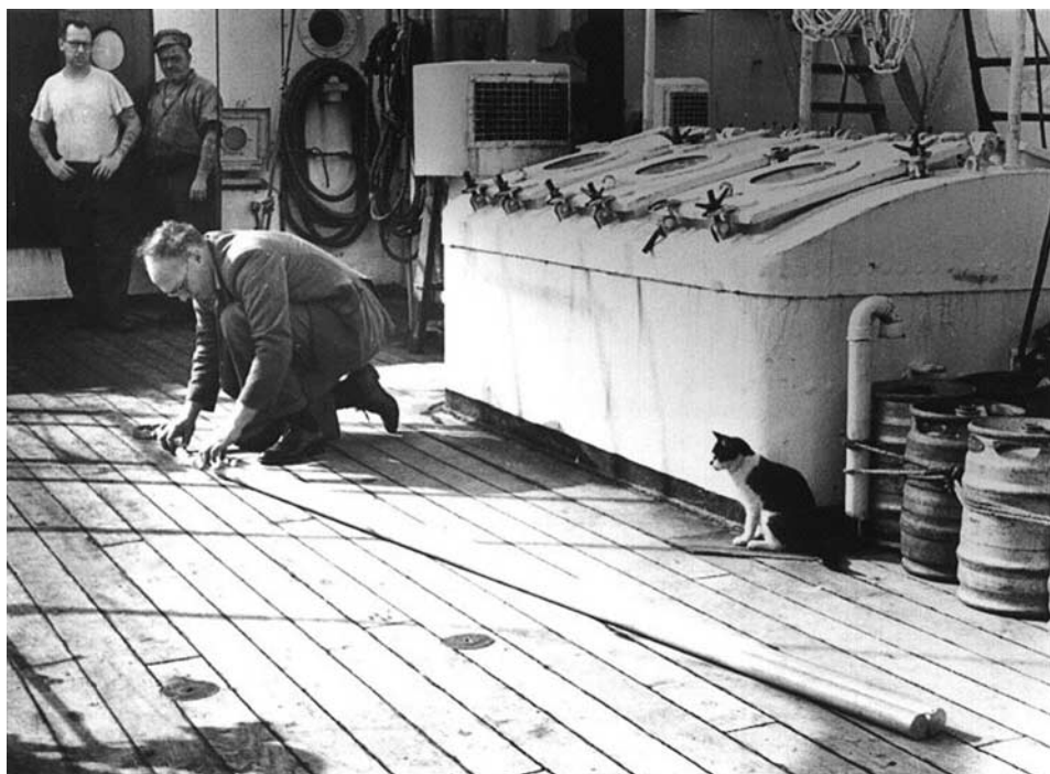
Figure 1.1 This widely reproduced photo shows John Swallow on deck preparing his float for launch. The float consisted of two aluminum tubes strapped together. The toroidal pinger (barely visible to Swallow's right) hangs underneath. Note the ship's cat paying close attention!
