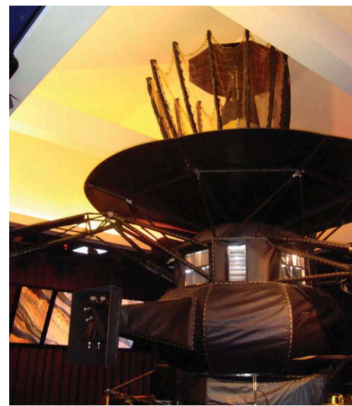
Figure 1.4 The Galileo engineering test model, on display at the Jet Propulsion Laboratory, Pasadena, CA. The wire mesh antenna at top is shown in its real-life jammed configuration.
