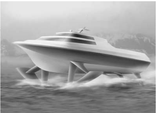
Figure 1.7. Hydrofoil vessel with free surface–piercing foils. (Artist: Bjarne Stenberg)
