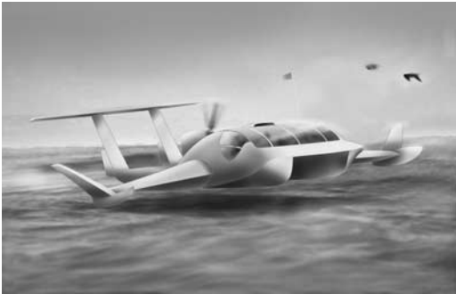
Figure 1.11. Artist’s impression of a WIG vehicle based on the Hoverwing technology by Fischer-Flugmechanick. An air-cushion effect is generated between the floats during takeoff. (Artist: Bjarne Stenberg)
