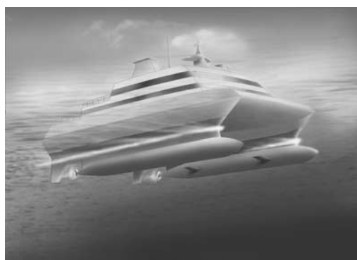
Figure 1.2. SWATH (small waterplane area twin hull). (Artist: Bjarne Stenberg)
