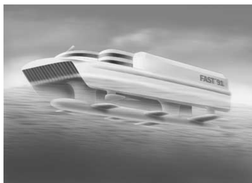
Figure 1.1. Fictitious high-speed vessel with air cushion, foils, and SWATH effects. (Artist: Bjarne Stenberg)
