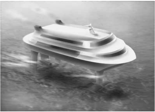
Figure 1.6. Hydrofoil vessel with fully submerged foil system. (Artist: Bjarne Stenberg)
