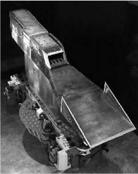
Figure 1.5. The rectangular engine configuration used for the National Aerospace Plane Program’s concept demonstration engine mounted atop its pedestal and the six-component force measurement system in preparation for testing in NASA Langley’s 8-ft. high-temperature tunnel.
