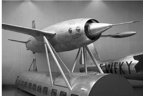
Figure 1.3. Leduc 0.10 at Musee de l'Air et de l'Espace at Le Bourget, France. The aircraft used a ramjet engine, and it was mounted on top of Languedoc aircraft for launch in flight.
