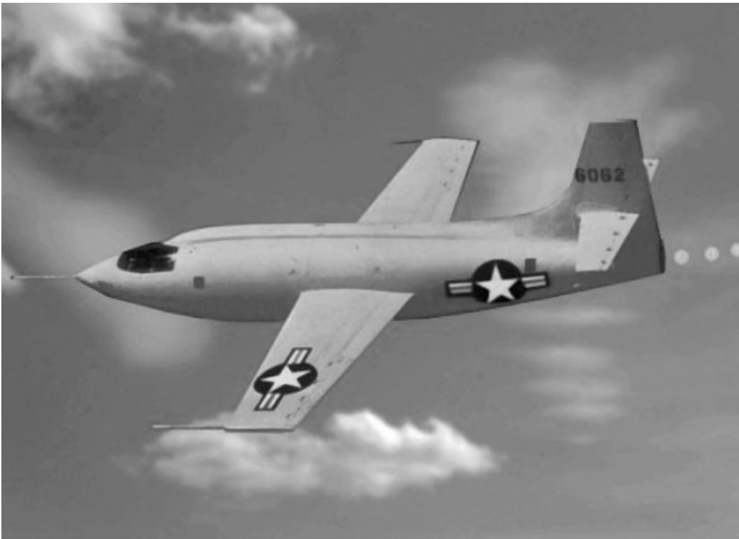
Figure 1.7. Bell XS-1: First supersonic airplane.
