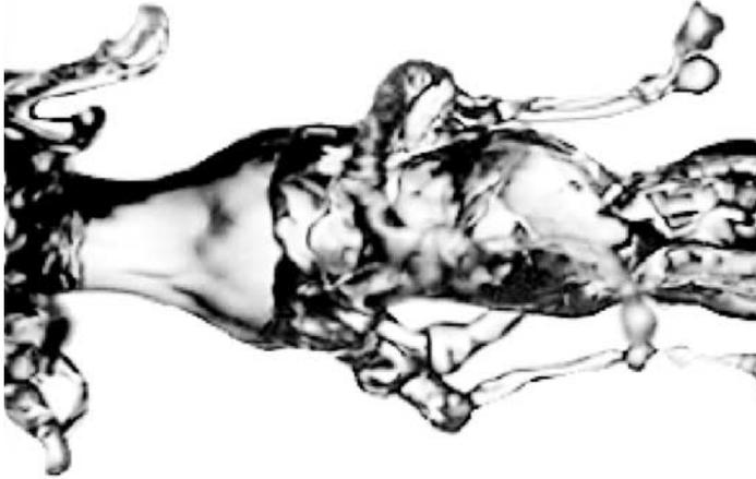
Fig. 1.2. A photograph of an atomization experiment performed with coaxial water and air jets reproduced from Villermaux *et al.* (2004). Reproduced with permission. Copyright American Physical Society.
