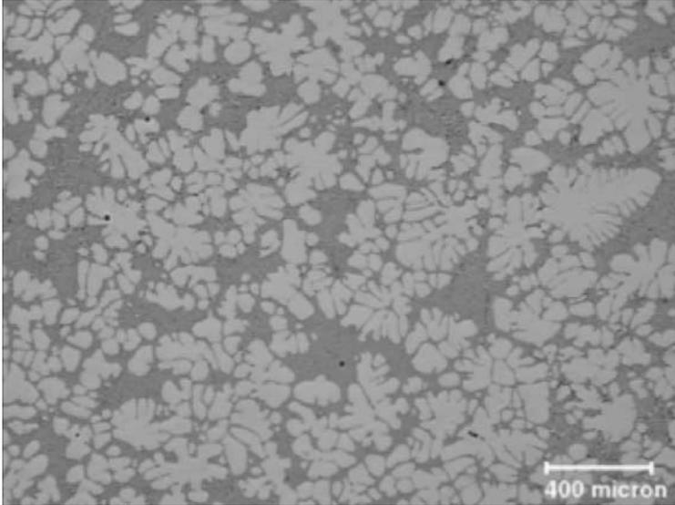
Fig. 1.5. Microstructure of an aluminum–silicon alloy. From D. Apelian, Worcester Polytechnic Institute. Reproduced with permission.
