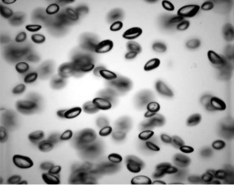
Fig. 1.1. A picture of many buoyant bubbles rising in an otherwise quiescent liquid pool. The average bubble diameter is about 2.2 mm and the void fraction is approximately 0.75%. From Bröder and Sommerfeld (2007). Reproduced with permission.
