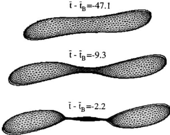
Fig. 1.7. A Stokes flow simulation of the breakup of a droplet in a linear shear flow. The barely visible line behind the numerical results is the outline of a drop traced from an experimental photograph. Reprinted with permission from Cristini *et al.* (1998). Copyright 2005, American Institute of Physics.
