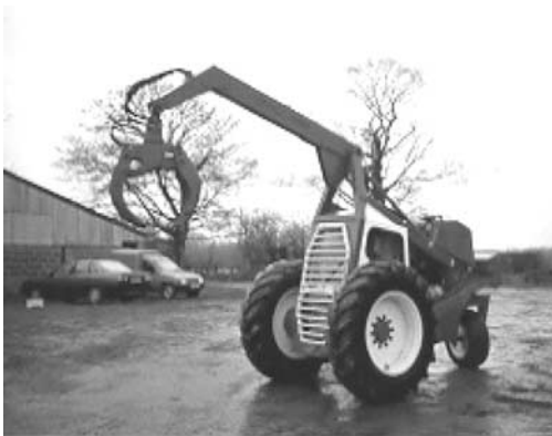
(a) A low-cost loader co-designed by the author, HR Wright, and Compact Loaders Ltd., the UK manufacturer
