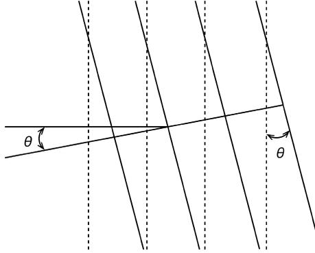
Figure 1.3. Approach of light wavefronts to an image plane.
