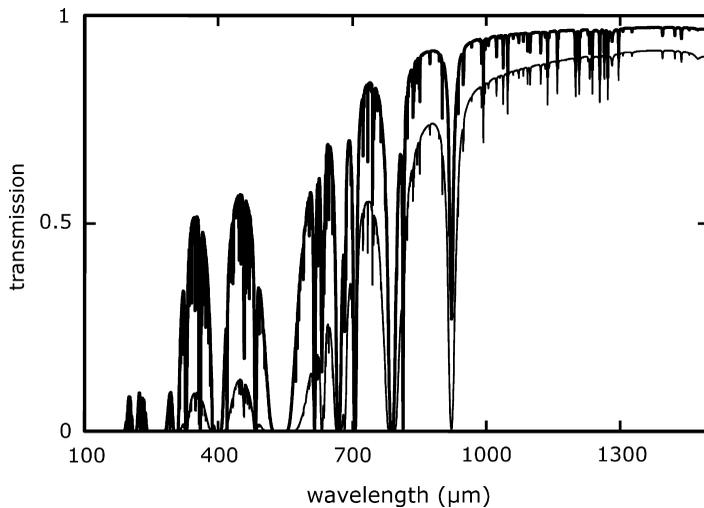
Figure 1.6. Atmospheric transmission in the submillimeter, for precipitable water vapor levels of 0.5 (heavy line) and 2 mm (light line). Prepared using APEX transmission calculator.
