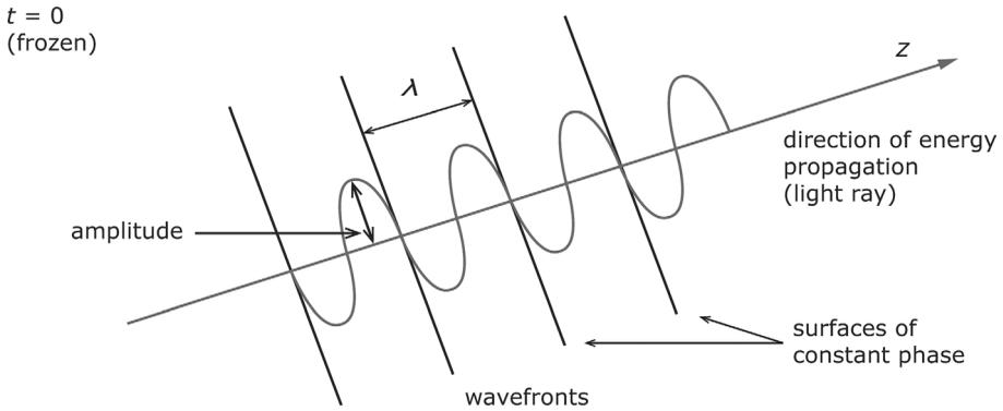
Figure 1.2. Terms describing the propagation of a photon, or a light ray. Redrawn with modifications from Barbastathis (2004).
