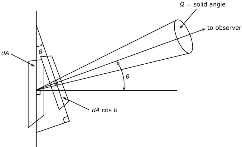
Figure 1.1. Emission geometry from a radiation source.
