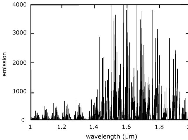
Figure 1.8. Sky brightness from 1 to 2  $\mu\text{m}$ . The vertical scale has been made 100 times larger than in Figure 1.7. Based on Rousselot *et al.* (2000).
