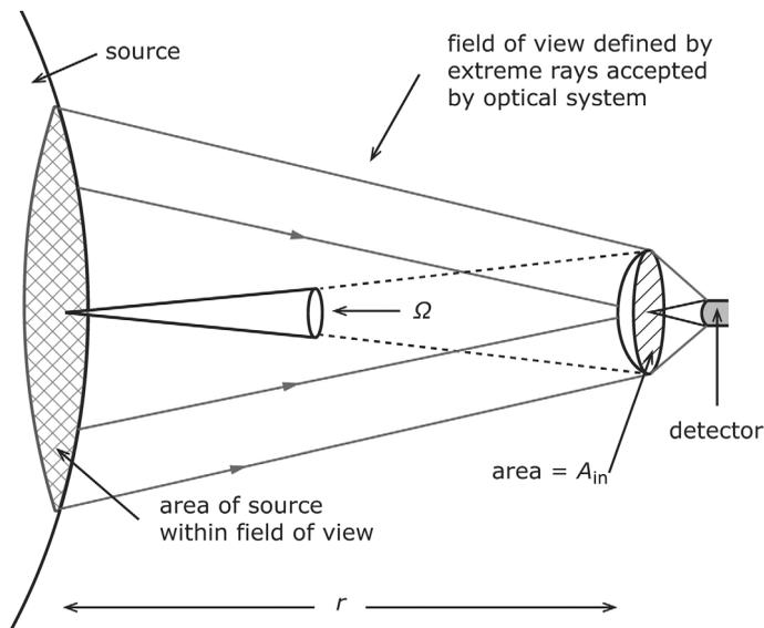
Figure 1.4. Geometry for detected signals.
