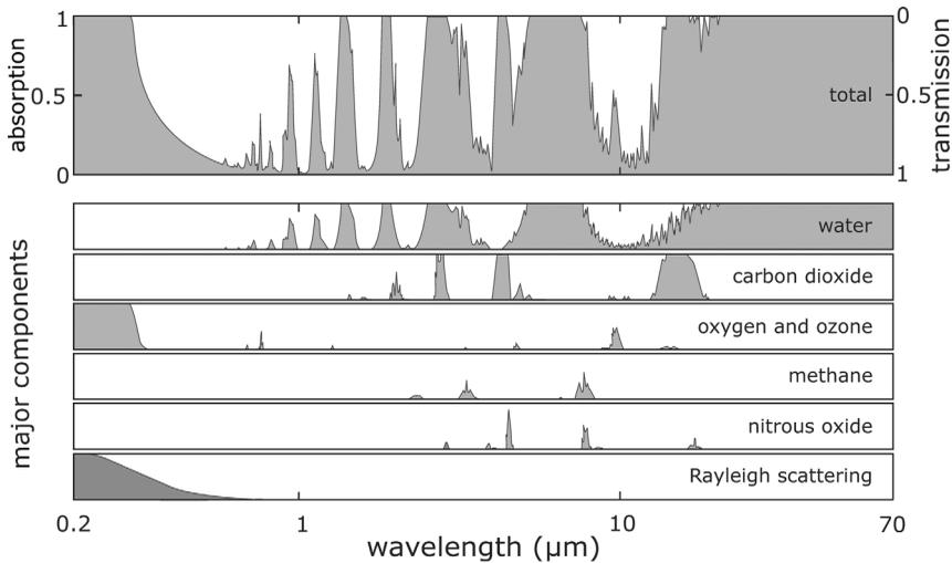
Figure 1.5. Atmospheric absorption and scattering. Redrawn with modifications from R. Rohde (n.d.).
